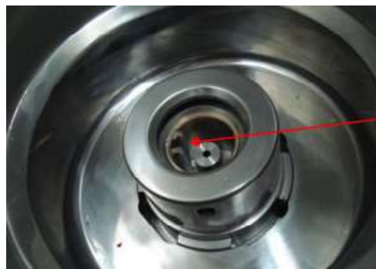
Grease cup: Lubricating grease injection device when bowl rotates
