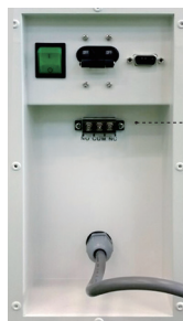
Alarm Signal Terminal 1 접점용 NO (Normal Open) COM (Common) NC (Normal Connect)
