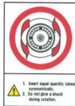
Symmetrical insertion of tubes caution warning
